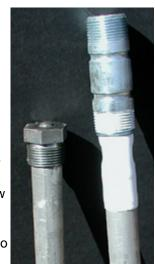
Standard hex-head anodes need 44 inches of overhead clearance. Standard combos need 48. Flexible anodes are loose links connected with flexible wire. They are good down to 12 inches overhead clearance, and can be cut shorter if they are too long for the tank.
